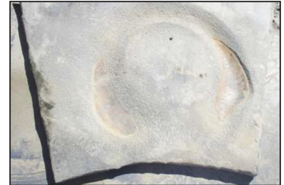
ARC coated wear plate after 30 days
